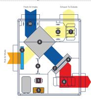
If the pool room air exceeds the maximum pre-set temperature, the Phoenix automatically increases the rate of introduction of cooler fresh air to help dissipate the excess heat.
