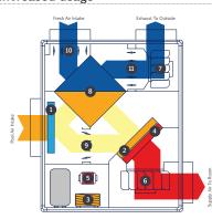
The Phoenix automatically increases introduction of dryer fresh air in line with the demand for humidity control. The expelled pool air is again first passed through the dehumidifying heat pump and then through the 'Cross Flow' multi-plate heat recuperator.
