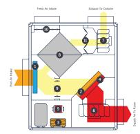
The Phoenix uses controlled fan power and the ability to re-circulate the pool room air to reduce ventilation to a minimum, saving unnecessary heat loss and electrical energy.
